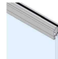
ISO glazing in thermally separated aluminium frame, double anti-burglary plastic glazing
